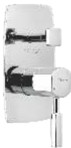
CS 1414SE Exposed part of single lever concealed diverter system consisting of operating lever and 2 mm thick sheet metal wall flange - without tip ton (suitable for CDC 103)
