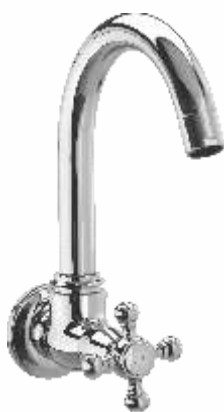
CQ 917 Sink cock (wall mounted) with 215 mm (8.5") long swivel spout and wall flange
