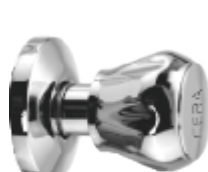
CQ 651E Quarter Turn CC 151E Half Turn Exposed part for flush cock 25 mm (1") consisting of operating lever, cartridge sleeve and wall flange (suitable for CFC 102)
