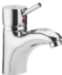
CQ 430 Single lever basin mixer with 450 mm braided connection pipe and provision for pop-up
