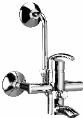
CS 912B Single lever wall mixer with 212 mm (8.5") max long bend pipe for overhead shower with built-in non return valve
