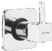
CS 427E Exposed part of concealed stop cock consisting of fitting sleeve, operating lever and adjustable wall flange (suitable for CSC 153 & CSC 202)
