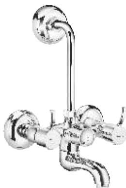
CQ 812B Wall mixer with 210 mm (8.5") max. long bend pipe for overhead shower with built-in non return valve
