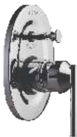
CQ 334E Exposed part of 5-way single lever concealed diverter system consisting of operating lever and wall flange - without tip ton (suitable for CDC 501)
